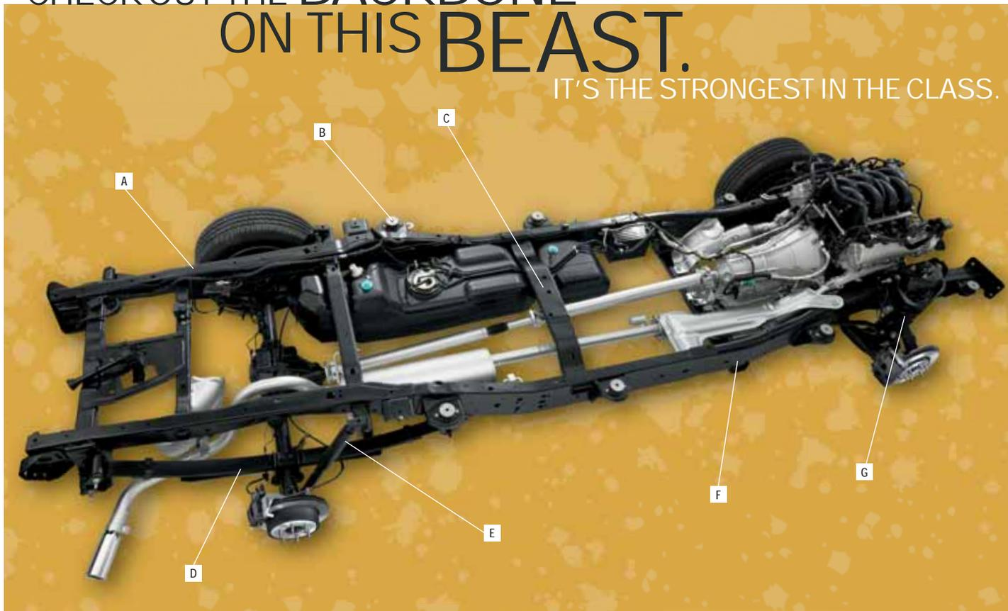
**STRONGEST FRAME IN THE CLASS (A)** is the backbone of F-150's class-leading capabilities. The fully boxed, ladder-style frame also contributes to the quiet interior and controlled ride.
