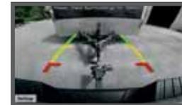
reverse for a wide-angle view behind the truck. The video display's built-in distance guide is ideal for trailer hookups.
