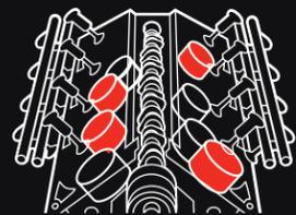
The 5.7-liter HEMI® with Variable Valve Timing (VVT) V8 Multi-Displacement System (MDS) brings fuel economy<sup>[1]</sup> to HEMI power. MDS allows the 5.7-liter HEMI VVT V8 engine with MDS — sporting best-in-class<sup>[2]</sup> 368 horsepower and 395
