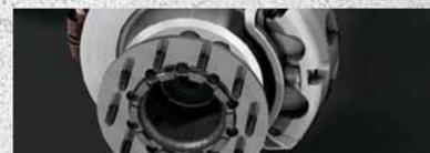
**A BRAKE SYSTEM THAT'LL STOP YOU IN YOUR TRACKS.** Ram 4500 and 5500 Chassis Cabs incorporate the largest front and rear brake rotors in their class,\* providing exceptional stopping power. Extra-large front and rear brake rotors measure over 15 inches in diameter, and the calipers are proportionally huge, featuring twin 66-mm pistons.
