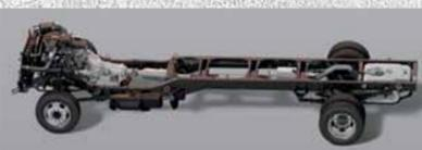
**PROVEN STRENGTH, SMART DESIGN.** Tested and rated to 50,000 psi, the frames for Ram Chassis Cabs carry their weight and more! Clean, flat frame rails, and a DEF system that is packaged out of upfit zones provide Ram Chassis Cabs with the backbone you need to get the job done. Add a largest-in-class\* 52-gallon rear fuel tank for increased up-time, and Ram Chassis Cab keeps you on the road for the long haul.
