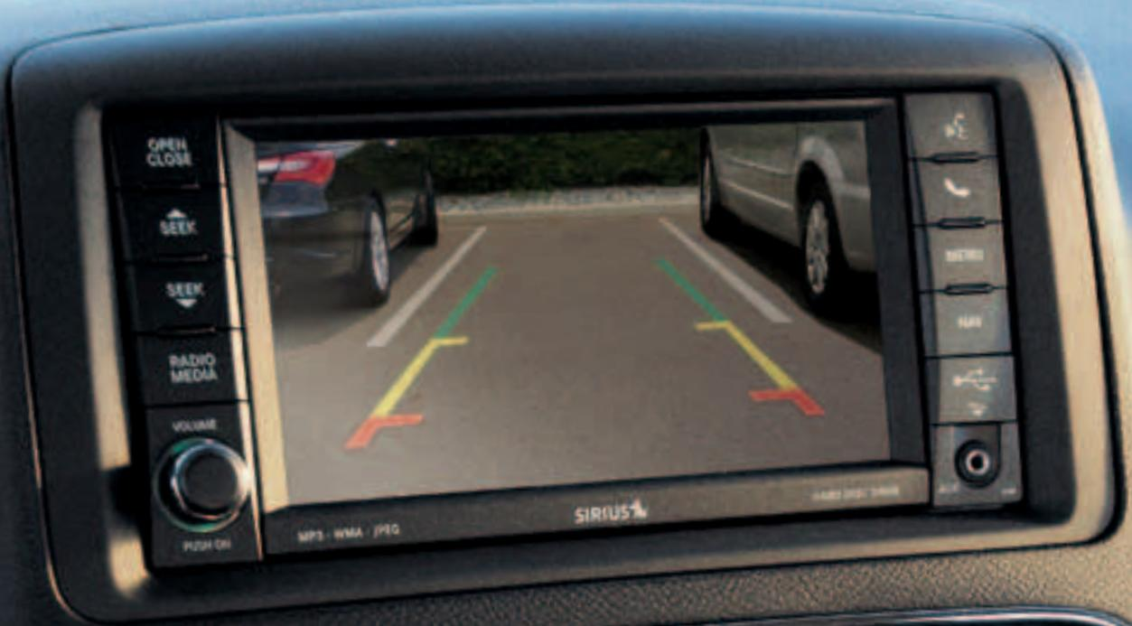
**PARKVIEW® REAR BACK-UP CAMERA.**<sup>(3)</sup> This standard system displays an accurate visual reference through your Uconnect® Media Center screen of what is behind your vehicle when driving in Reverse. It includes new on-screen static guidelines to help orientate the driver while backing up.
