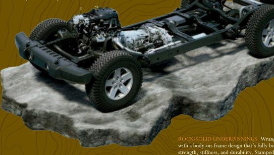
ROCK-SOLID UNDERPINNINGS. Wrangler is built with a body-on-frame design that's fully boxed for strength, stiffness, and durability. Stamped steel skid plates for fuel tank, transfer case, and automatic transmission oil pan, if equipped, help protect Wrangler's guts when battling boulders. Extra-tough body-mounted rails provide additional protection (standard only on Rubicon).
