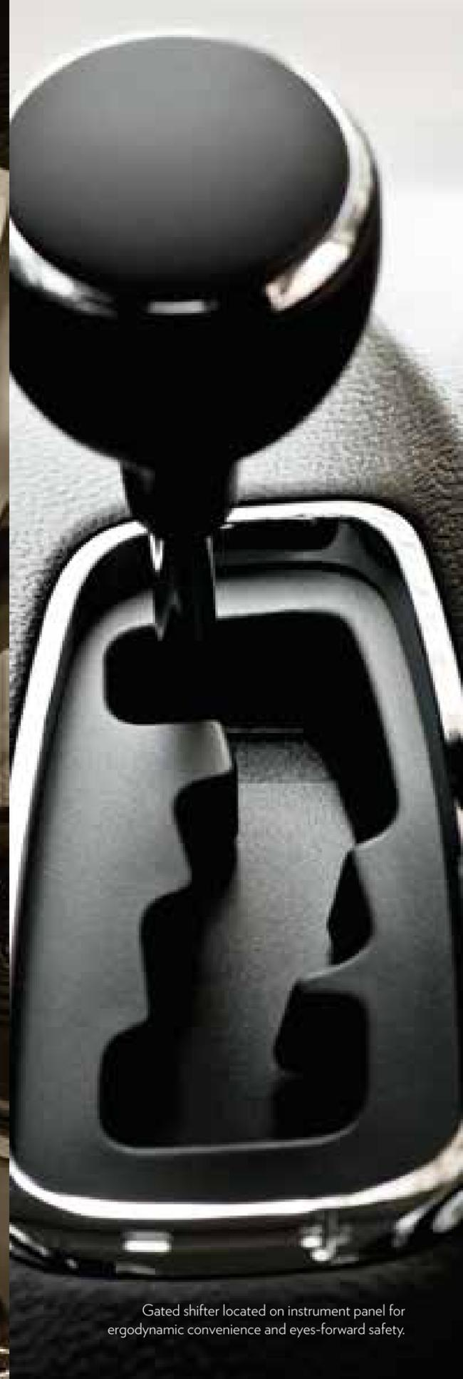
Gated shifter located on instrument panel for ergonomic convenience and eyes-forward safety.
