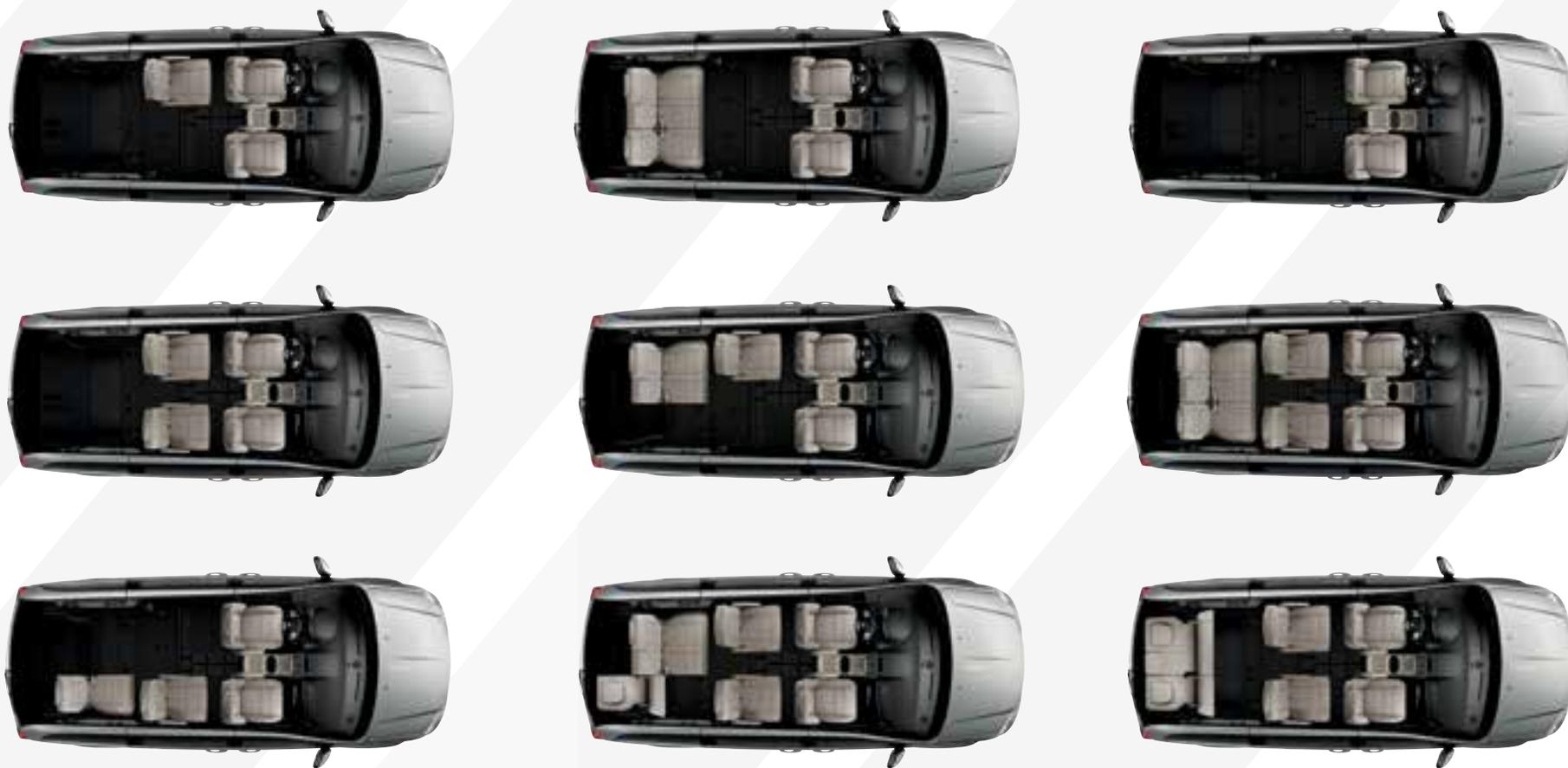
Whether it's configuration one or 81, creating the perfect seating and cargo combination is quickly achieved without physically removing any seats from the interior. They're simply stowed in-floor. Go configure!
