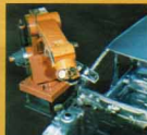
A programmed optic scanner checks openings around doors, windows, trunk lids and taillamps for accuracy.
