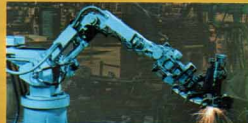
A robotic arc welding system makes spot welds quickly, precisely and automatically.
