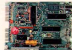
Computer Command Control helps reduce exhaust emissions while allowing good fuel efficiency.
