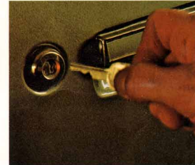
Illumination package. Lift handle, door lock is illuminated, interior lights go on.
