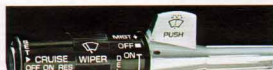
The all-in-one "smart stick" Controls windshield washers, wipers, high-beam lights, turn signals. Cruise Control available.
