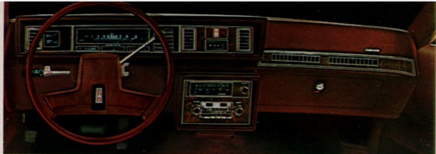
Cutlass Supreme instrument panel with wood grain vinyl and deluxe steering wheel.
