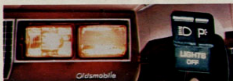
Headlamp-on reminder, standard. Sounds and flashes a warning when door is opened.
