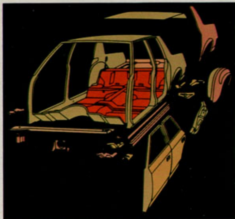
Extensive anti-corrosion measures. Includes galvanized metals, plastisols, sealers, front fender liners, waxes and zinc-rich primers.
