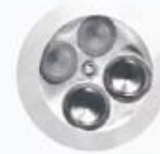
**Four-valve cylinder head.** Four valves per cylinder improve engine performance on the SL2 by allowing it to breathe more efficiently. And that, in turn, is easier on the environment. Saturn uses a lost-foam casting process for most major engine components to get higher quality castings with fewer parts and less machining, which leads to less waste.
