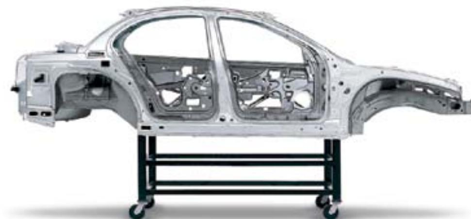
**Spaceframe construction.** Think of it as a protective cage that entirely surrounds the passenger compartment. This welded steel structure is an important reason for Saturn's performance in crash tests and in crash survival on the road. Steel door beams and cross bracing add side-impact protection. And there's an incidental benefit to the spaceframe: fewer rattles and squeaks down the road.
