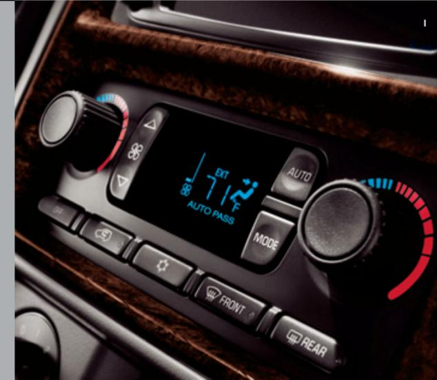
I. The automatic dual-zone climate control lets you dial in a difference of up to 25°F between driver and front passenger.
