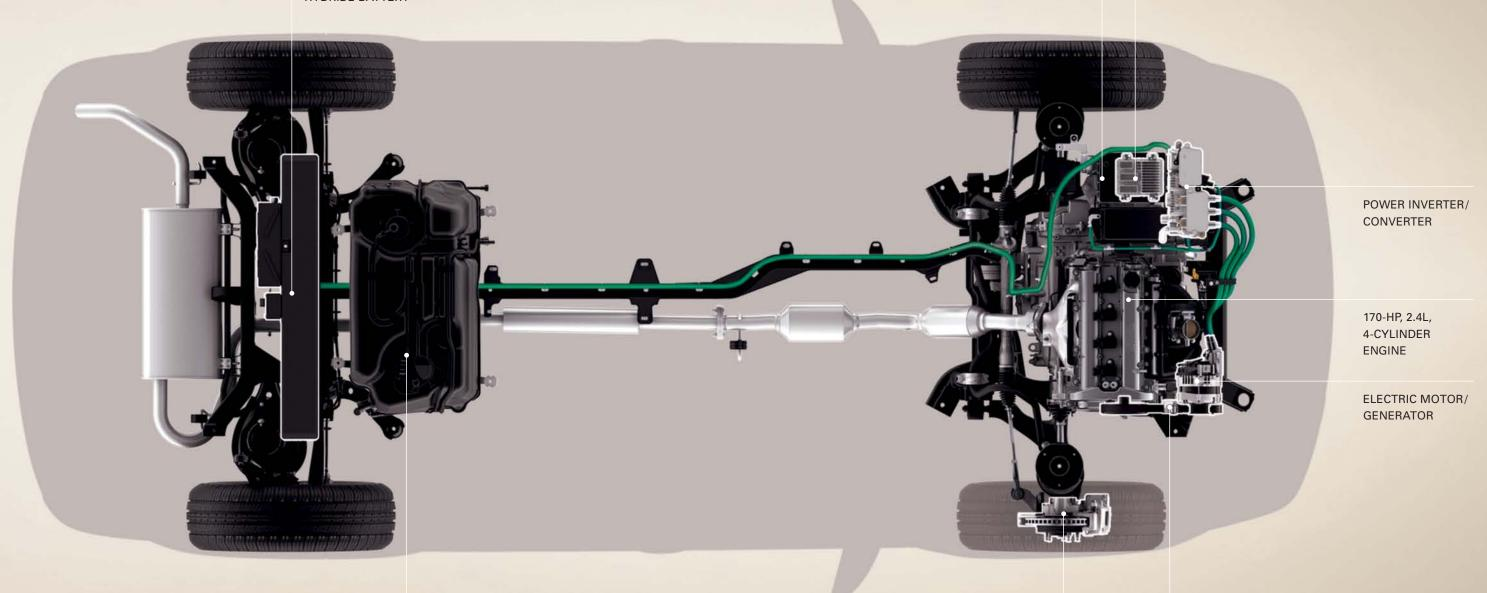
AT A COMPLETE STOP, the VUE Green Line's 36-volt battery powers the vehicle accessories, allowing the gas engine to shut off and save fuel.\*
