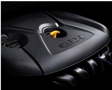
**ADVANCED ENGINE TECH** The Elantra's available 2.0-liter engine draws its responsive power from Gasoline Direct Injection (GDI) and Dual Continuously Variable Valve Timing. GDI atomizes fuel directly into each cylinder's combustion chamber for added power and greater fuel efficiency with cleaner emissions.
