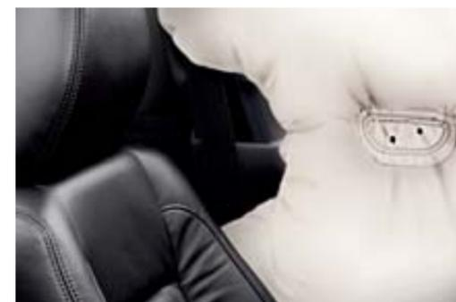
**Side-impact air bags** Mounted in the front seats to help provide the best protection no matter what your ideal seat position is. Designed to help protect both your head and torso, they helped the Forester achieve the highest crash-test safety scores in Insurance Institute for Highway Safety (IIHS) testing.<sup>3</sup>
