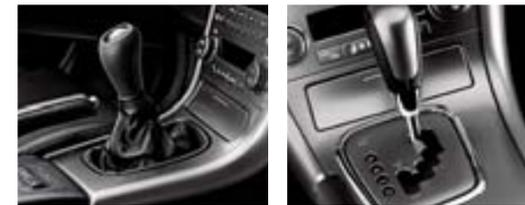
**5-speed manual transmission** It's fully synchronized for precise shifts. The Legacy 2.5 GT Limited has a reinforced dual-mass flywheel clutch for even smoother, direct action.
