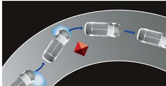
**Active safety** Lower center of gravity due to SUBARU BOXER engine • Symmetrical All-Wheel Drive stability • 4-wheel independent suspension • Responsive rack-and-pinion steering • Daytime Running Lights (DRL) • 4-wheel disc brakes • 4-channel, 4-sensor antilock brakes (ABS) • Electronic Brake-force Distribution (EBD)
