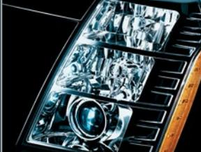
**IntelliBeam**, an available feature, turns the high-beams on automatically, and switches to low-beams when oncoming headlamps or taillamps are detected.
