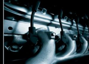
**A 403-horsepower 6.2L Vortec V8 engine** is an all-aluminum design with Variable Valve Timing and Active Fuel Management for improved fuel efficiency.<sup>4</sup>
