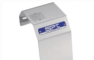
**Turbo Heat Shield.** The SPT Heat Shield works to retain heat within the turbocharger, helping to maintain turbocharger exhaust gas velocity. The shroud also helps keep heat generated by the turbocharger away from the intercooler.
