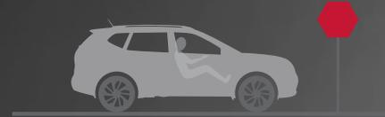
**Active Trace Control.** A turn for the better. This innovative technology helps improve control when you take a corner. It reads the cornering situation and, if needed, can brake each wheel individually to help you steer through the turn with confidence.
