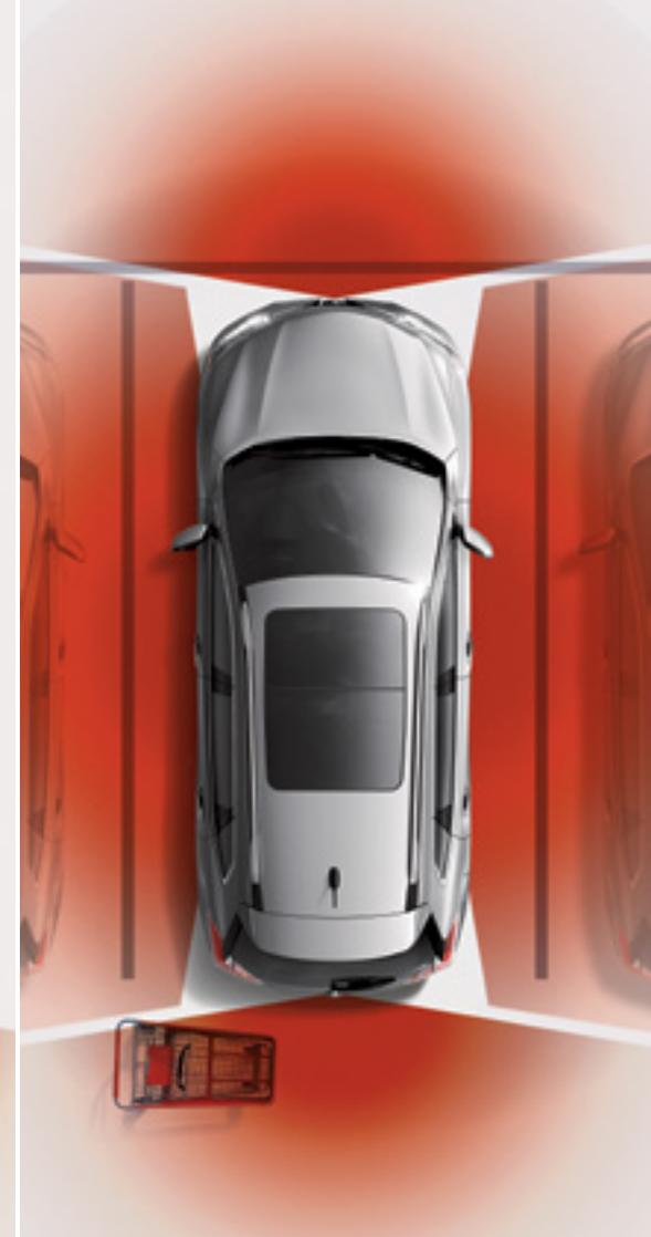
**Moving Object Detection.** When the Around View® Monitor is in use and detects something moving by the vehicle, it gives a visual and audible alert.<sup>5</sup>
