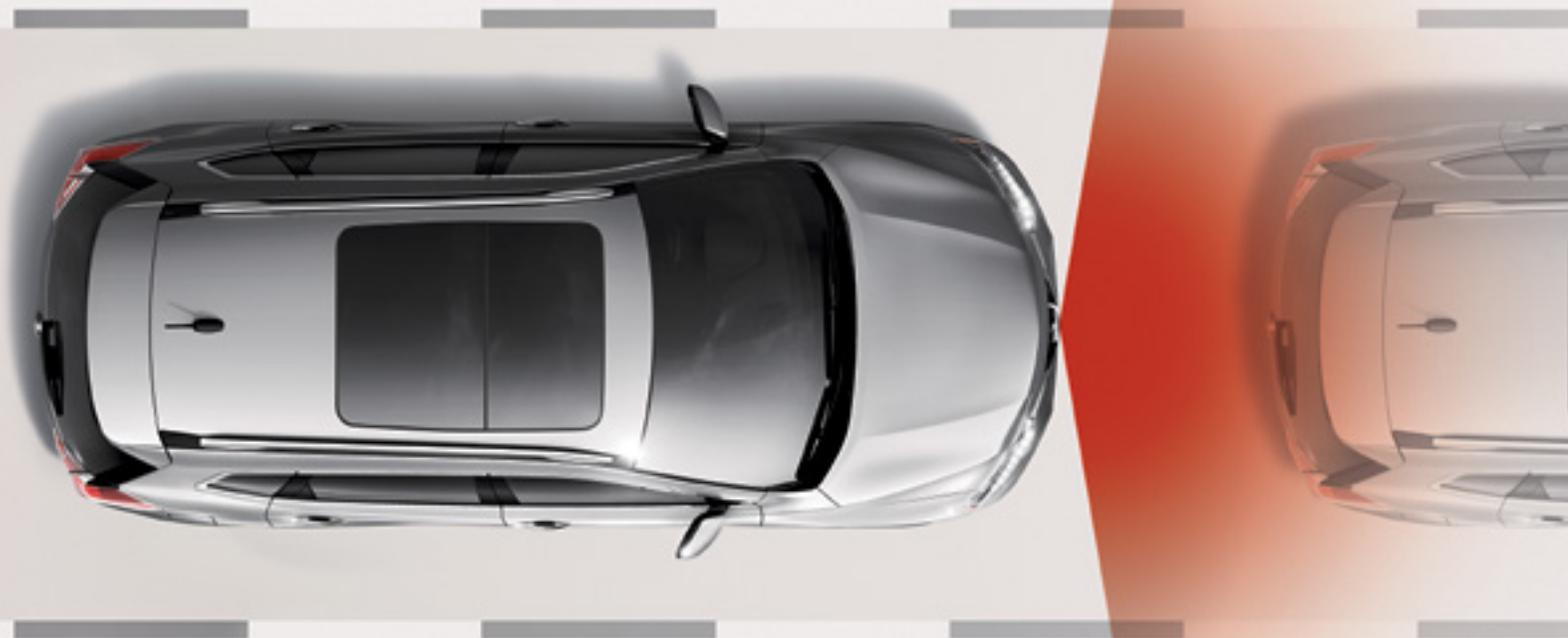
**Forward Collision Warning.** Whether it's rapidly slowing traffic ahead, or someone making a surprise merge into your lane, you can get caught off guard in a potentially dangerous situation. How about a little help? With Forward Collision Warning, a sensor on the front of Rogue® constantly monitors the vehicles ahead in your lane and, when the system detects a potential risk, gives you an audible warning and a visual signal on the instrument panel.<sup>2</sup>
