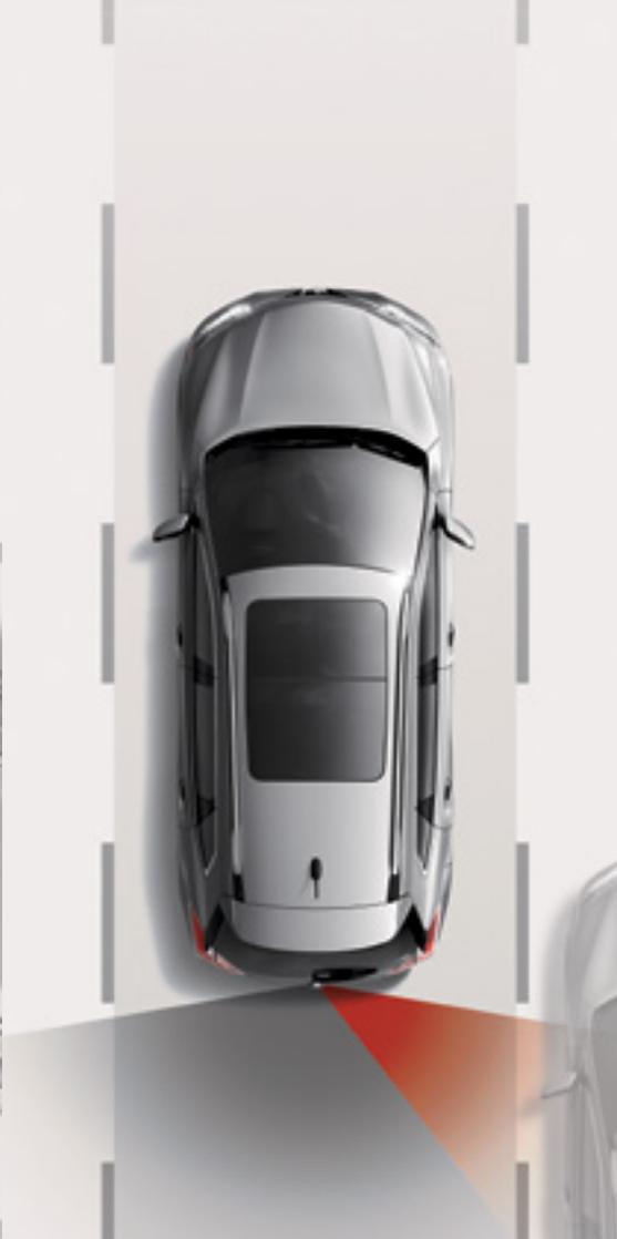
**Blind Spot Warning.** If another vehicle is detected in your blind spot area, an indicator appears in the driver's or front passenger's doors and on the Advanced Drive-Assist® Display. Put your turn signal on, and the indicator flashes with a warning chime to alert you.<sup>3</sup>
