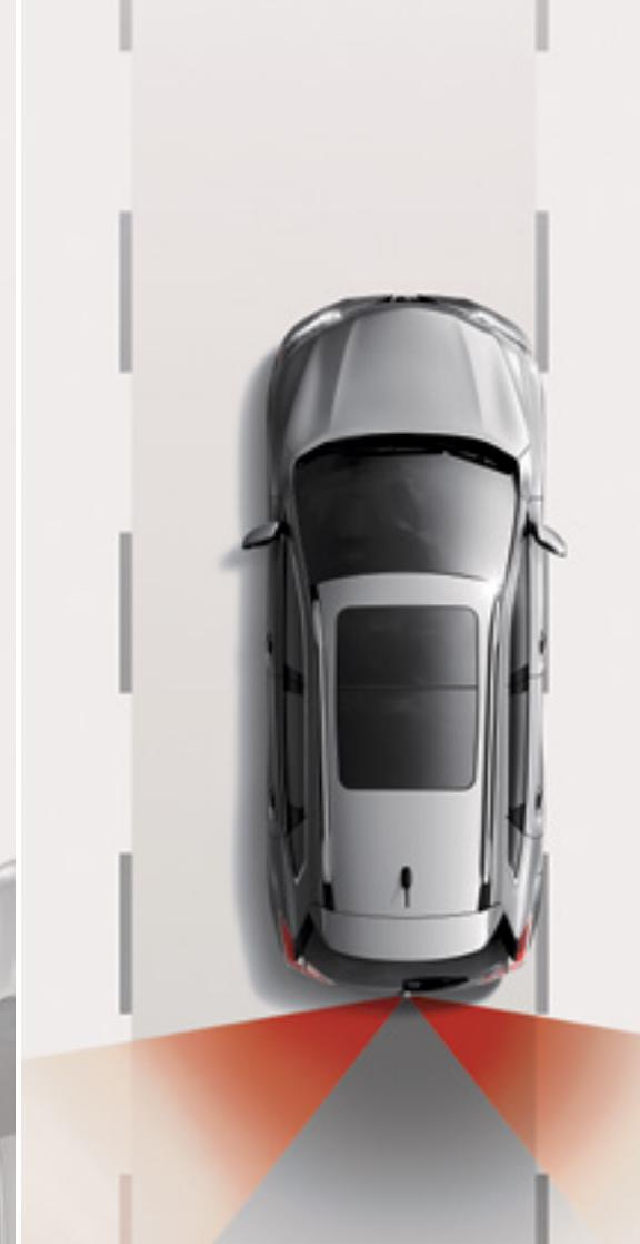
**Lane Departure Warning.** If Rogue® detects that you're straying from your lane, the Lane Departure Warning system will give both a visual and audible alert. The system is so smart, it's designed to stop the warnings whenever your turn signal is engaged.<sup>4</sup>
