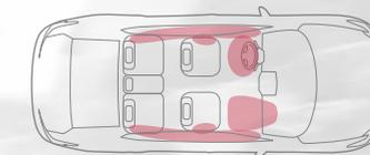
**6 Standard Air Bags.**<sup>10</sup> Nissan Advanced Air Bag System has supplemental front air bags with seat belt and occupant-classification sensors.<sup>10</sup> In addition, Maxima® features front seat-mounted side-impact supplemental air bags,<sup>10</sup> and roof-mounted curtain side-impact supplemental air bags with rollover sensor.<sup>10</sup>
