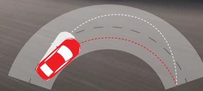
**Active Trace Control.** By selectively applying Maxima's® brakes when cornering, Active Trace Control can automatically engage the inner or outer brakes, helping to optimize your line through a turn.<sup>2</sup>
