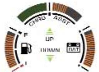
*Fuel supply and electrical energy capacity, including state-of-charge, are displayed on the right side of the Electronic Instrument Display.*
