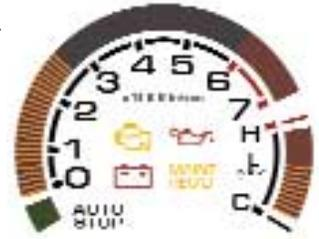
*The Insight's Electronic Instrument Display is logical and easy to read: on the left is engine status information, such as rpm and engine coolant temperature.*
