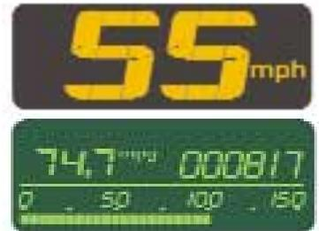
*The middle of the Electronic Instrument Display provides a wealth of information, including present speed, the distance the car has traveled, and both current and cumulative fuel economy.*
