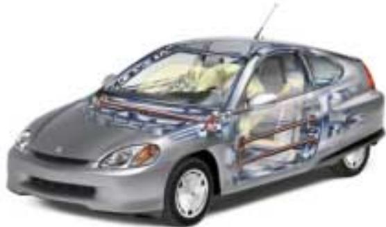
*Crumple Zones built into the Insight's highly rigid aluminum body are designed to help protect the driver and passenger in an impact.*
