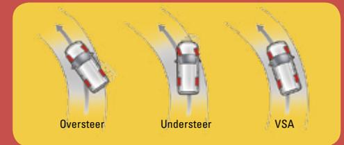
Vehicle Stability Assist (VSA) can help detect oversteer or understeer, to help restore the driver's intended path.
