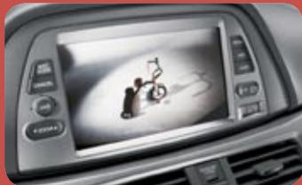
On models equipped with navigation, the screen doubles as a full-color rearview camera display, giving you a clear view of the area directly behind the vehicle when you shift into reverse. New for 2008, EX-L models without navigation show the image on a camera display located in the rearview mirror.
