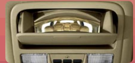
The Odyssey's large power moonroof on EX-L and Touring models features a tilt function as well as an air diffuser to let air circulate inside the cabin without causing too much turbulence.
