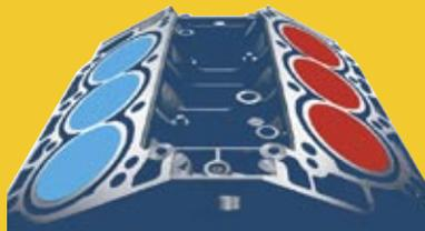
During steady cruising, the Odyssey's V-6 shuts down the entire rear bank of cylinders. An Active Noise Cancellation™ (ANC) system helps control engine noise.
