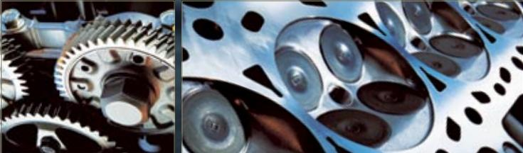
THE S2000'S ENGINE IS SURPRISINGLY COMPACT CONSIDERING ITS POWER OUTPUT. THIS IS ACHIEVED WITH TECHNOLOGY LIKE A NARROW DOHC DESIGN WITH A SPACE-EFFICIENT SILENT-CHAIN PRIMARY DRIVE AND GEAR-DRIVEN SECONDARY DRIVE.
