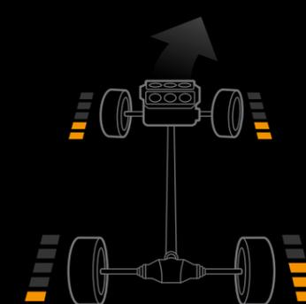
For increased stability during lane changes, the SH-AWD system transfers power to the inside rear wheel.
