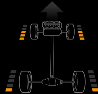
For better fuel efficiency, up to 90% of the power is sent to the front wheels when cruising in a straight line.
