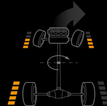
When cornering on dry surfaces, up to 70% of the torque is distributed to the rear. Torque vectoring allows up to 100% of the power to distribute to the outside rear wheel, improving control and helping rotate the TLX through the turn.
