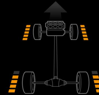
As weight shifts to the rear of the TLX during hard acceleration, the SH-AWD system transfers up to 44% of the power to the rear wheels to take advantage of available traction.
