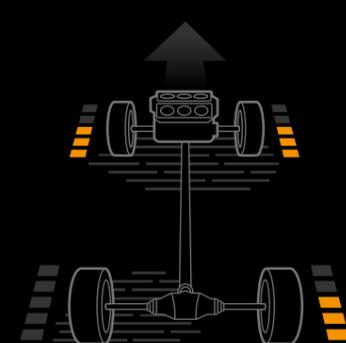
Under slick conditions, SH-AWD actively sends power to the wheel with the most traction.
