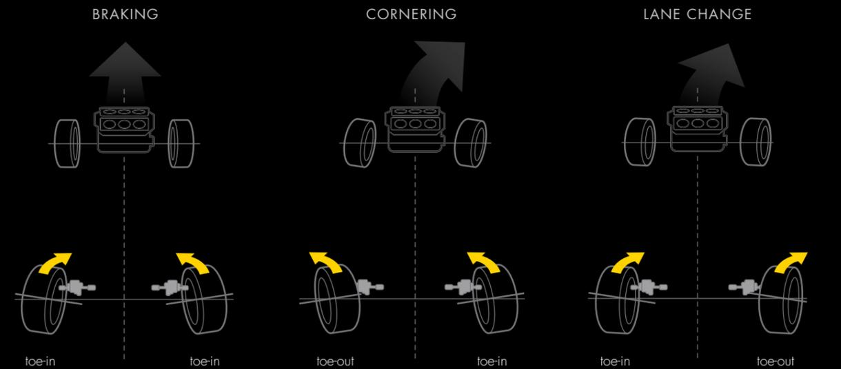
While braking, each rear wheel adjusts inward, increasing stability.
