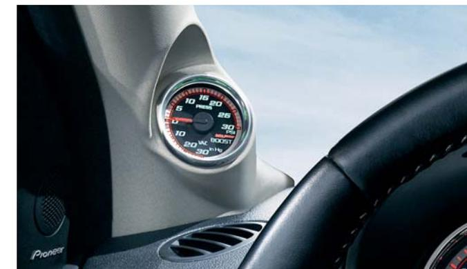
SS Turbocharged models include an A-pillar-mounted boost gauge.
