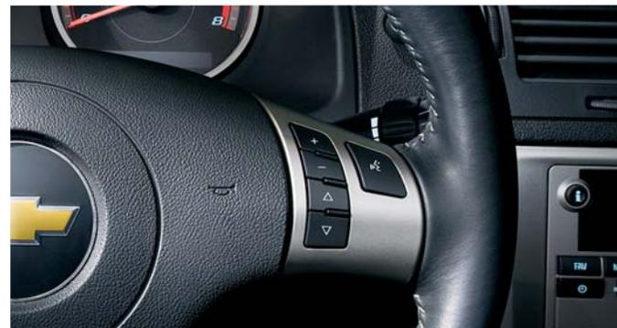
Steering wheel-mounted audio and cruise controls.
