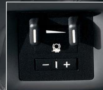
**THE AVAILABLE TRAILER BRAKE CONTROLLER** comes with instrument panel-mounted controls. It's integrated with the ABS to provide immediate and measured brake force signaling to electrically controlled trailer brake systems.
