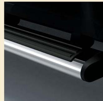
**OVAL ASSIST STEPS** make it easier to get into and out of your Silverado. These stylish six-inch-diameter, high-strength, corrosion-resistant, stainless steel oval assist steps are available in Black or chrome.
