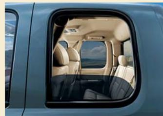
**FULL-DROP POWER REAR WINDOWS** are standard in Extended Cab LT and LTZ models. These large rear windows power down completely into the rear doors at the touch of a button for added comfort and convenience.
