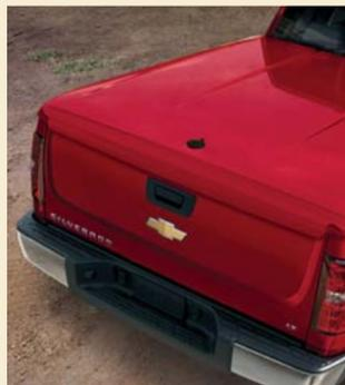
**A HARD COMPOSITE TONNEAU COVER** features struts for easy opening and closing, a lock and a quick-release mechanism for easy removal.
