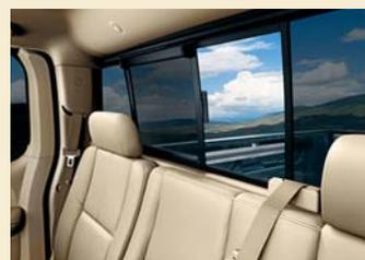
**THE POWER SIDE-SLIDING REAR WINDOW** enhances your driving comfort. Operated with a switch in the upper console, this available window slides sideways from the center position to the passenger side.
