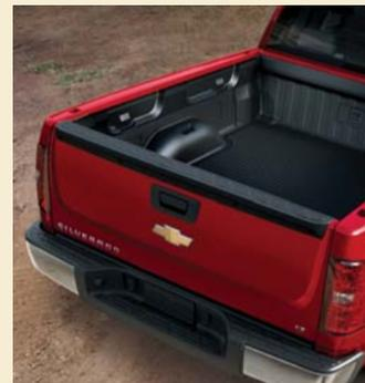
**THE BEDLINER AND TAILGATE LINER** are made of black, high-density, skid-resistant polyethylene.<sup>1</sup>
