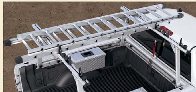
**THE CARGO MANAGEMENT SYSTEM** can support up to a 500-lb<sup>1</sup> load. The rear rack slides along the rails and includes four load stops.
