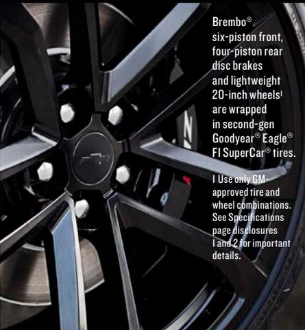
Brembo® six-piston front, four-piston rear disc brakes and lightweight 20-inch wheels<sup>1</sup> are wrapped in second-gen Goodyear® Eagle® F1 SuperCar® tires.
