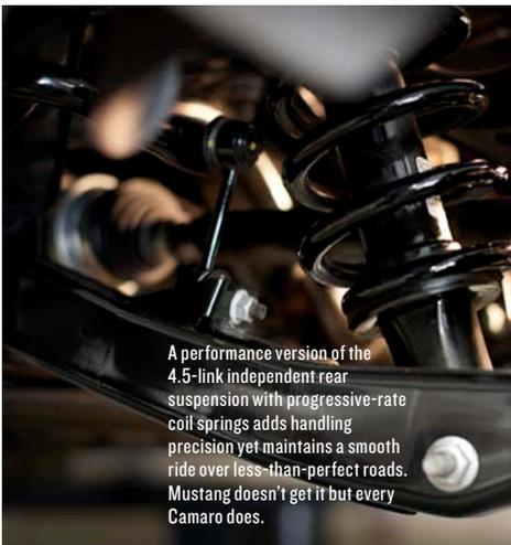
A performance version of the 4.5-link independent rear suspension with progressive-rate coil springs adds handling precision yet maintains a smooth ride over less-than-perfect roads. Mustang doesn't get it but every Camaro does.
