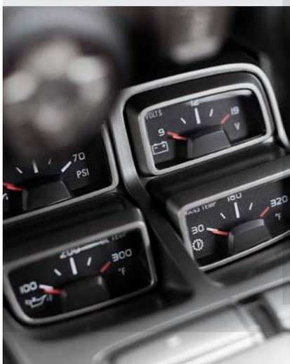
A four-pack of auxiliary gauges—standard on 2LT and 2SS—includes oil pressure, oil temperature, transmission temperature and voltmeter.
