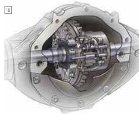
**10 EATON AUTOMATIC LOCKING REAR DIFFERENTIAL** When the available Eaton locker senses a difference in wheel speed between the left and right rear wheels of approximately 100 rpm, it locks both to turn in unison for added traction.
