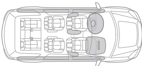
**SIDE-IMPACT AIR BAGS<sup>1</sup>** They are mounted on the driver and front-passenger seats to help protect the thorax and pelvic regions of the driver and front passenger in a side-impact collision.
