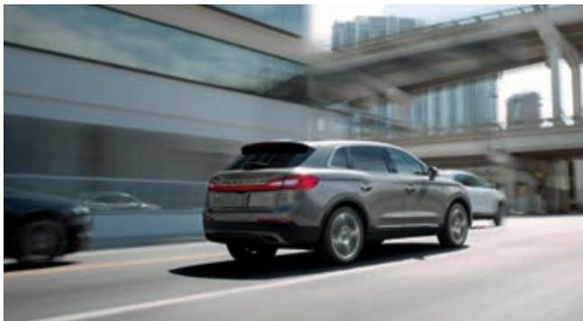
**BLIS® (BLIND SPOT INFORMATION SYSTEM) WITH CROSS-TRAFFIC ALERT<sup>1,2</sup>** – Some vehicles may be out of your line of sight, but they can be detected by this technology. It warns you if it detects a vehicle in your blind spots while driving forward, or approaching from the sides while in Reverse.
