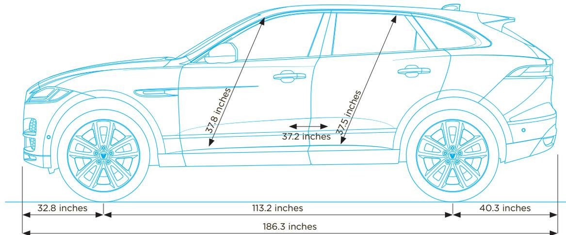
Dimensions were measured with vehicle at unladen weight
