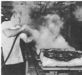
The rich wool broadcloth upholstery of an Imperial seat unit is not only meticulously fitted by expert tailors, but is steam shrunk to the seat so it will not sag or pull out of shape.
